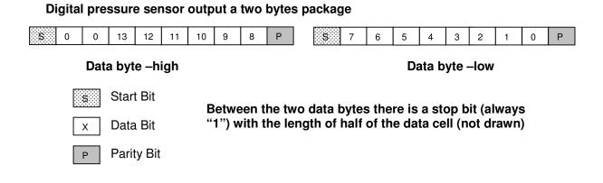
The transmission speed depends on the update rate and ranges up to 8 KHz.
