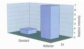
An optimized reflector design offers a gain of approx. 7 times in intensity on the optical axis.
