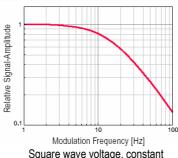
Square wave voltage, constant amplitude 50% duty cycle.
